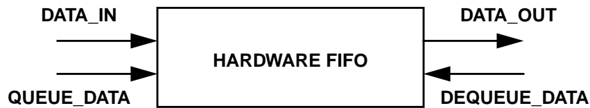
Figure 2.19 An interface model of a hardware FIFO.
