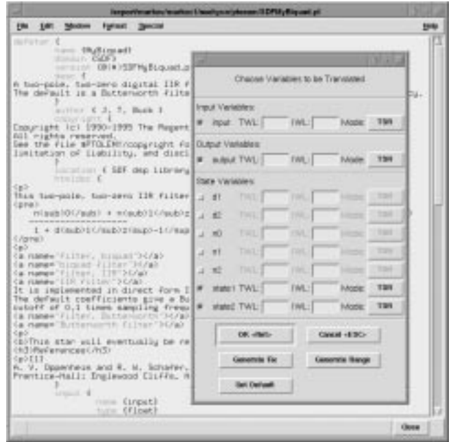
Fig. 1. A ptlang description for a biquad filter and a dialog box querying the user to select ports and states to be examined.
