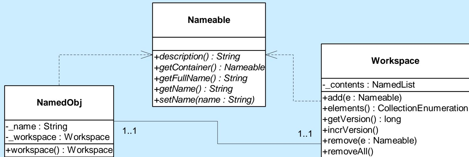
Every **NamedObj** has an immutable association with an instance of **Workspace**. A monitor on **Workspace** is used for thread synchronization, and the workspace tracks versions of a topology.
