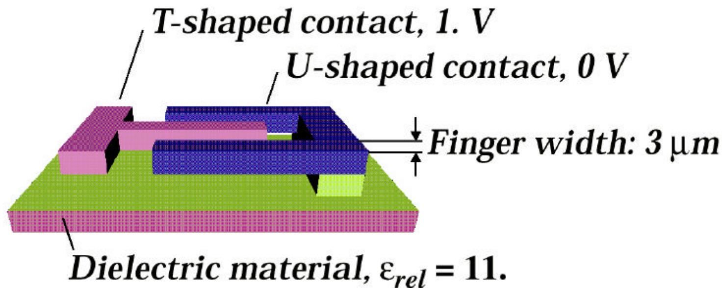
We have incorporated a macro-model of a mechanical comb constructed by Coyote using their electrostatic BEM method.
