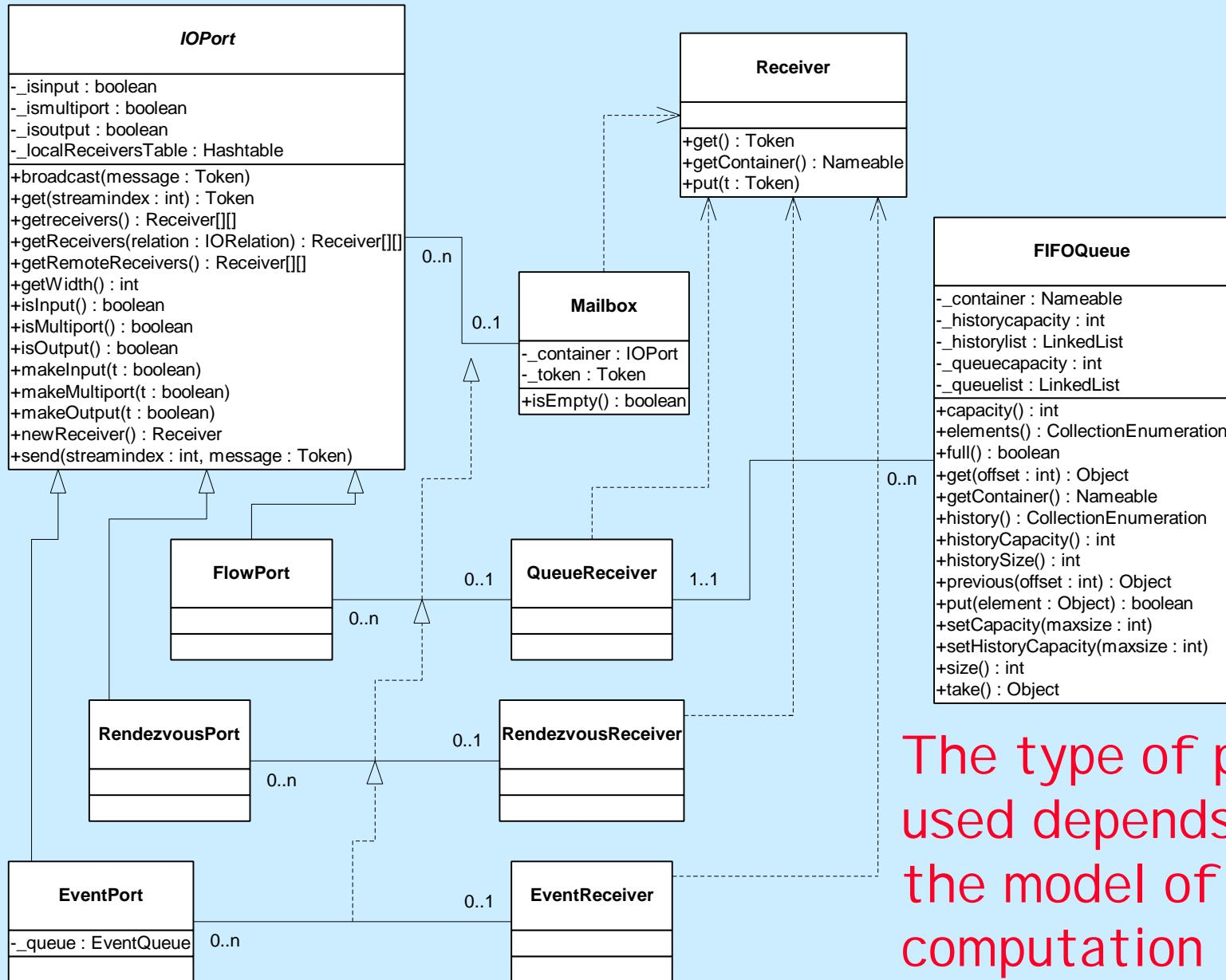
The type of port used depends on the model of computation
