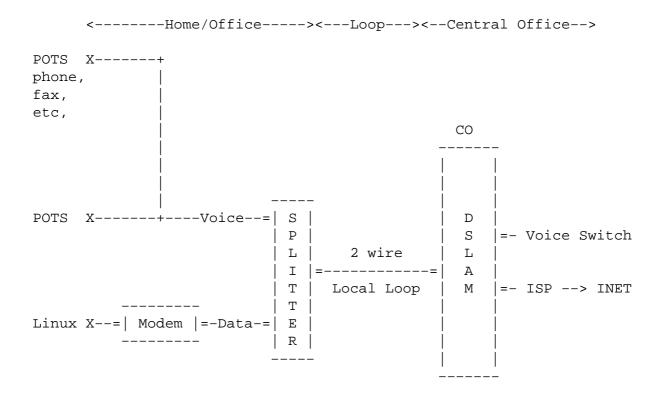
Figure 2: DSL Splitterless (a.k.a. filtered) Block Diagram
