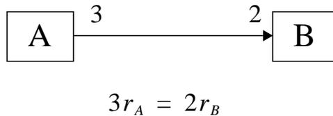
**Figure 10. A simple SDF graph and its balance equation.**
