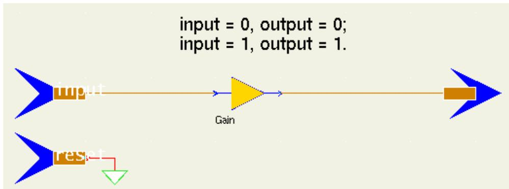
Figure 22. The SDF galaxy associated with the State0 state in the 1-bit counter.
