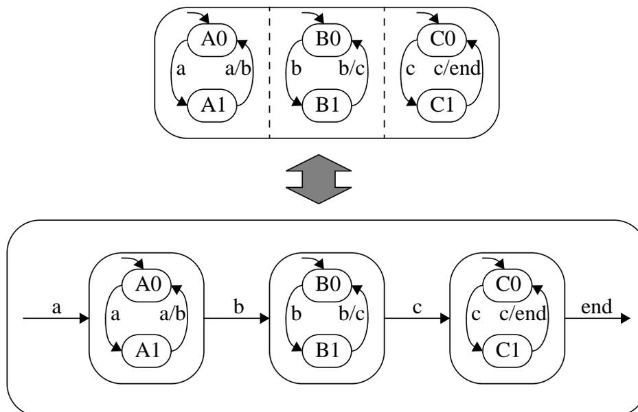
**Figure 5. The specification of concurrent FSMs in Statecharts can be considered as a syntactic shorthand for an interconnection of FSMs in a concurrency model.**
