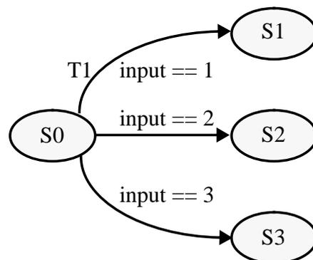
Figure 13. When the input is equal to one, this FSM makes a transition from S0 to S1.
