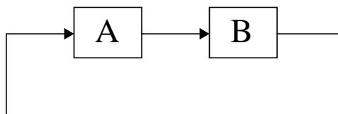
Figure 12. An SDF graph with a zero-delay loop.
