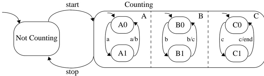
Figure 2. An HFSM representation of a 3-bit counter.
