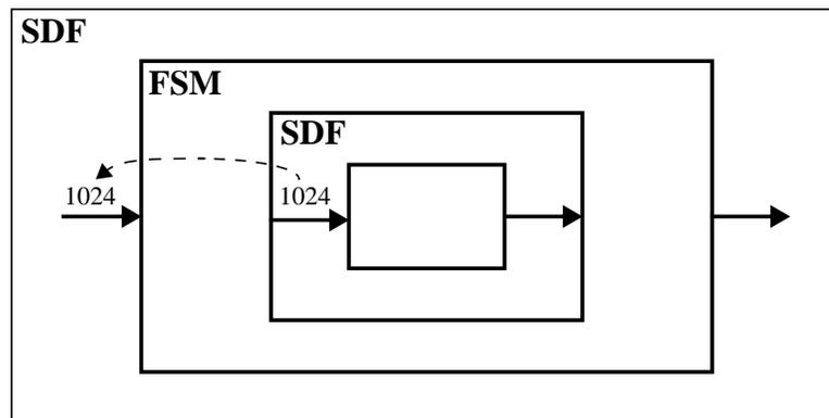
**Figure 16. If an SDF subsystem is embedded in an FSM which is inside another SDF domain, the FSM will inform the outer SDF domain how many tokens are consumed at the input of the inner SDF subsystem.**
