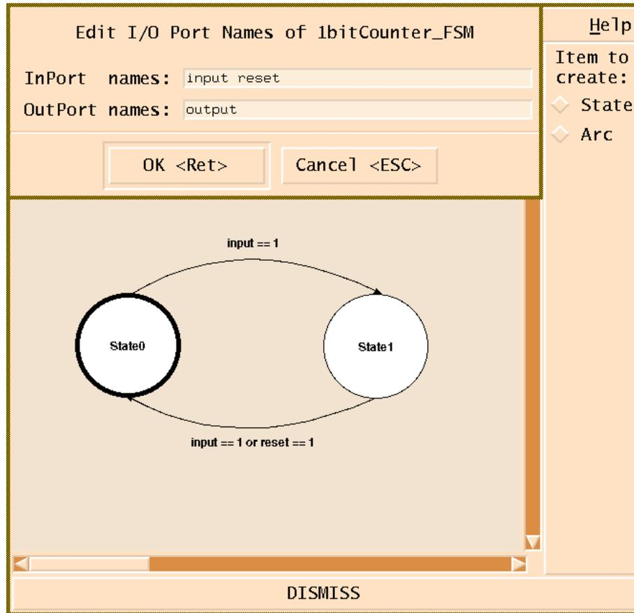
Figure 21. The FSM of the 1-bit counter.
