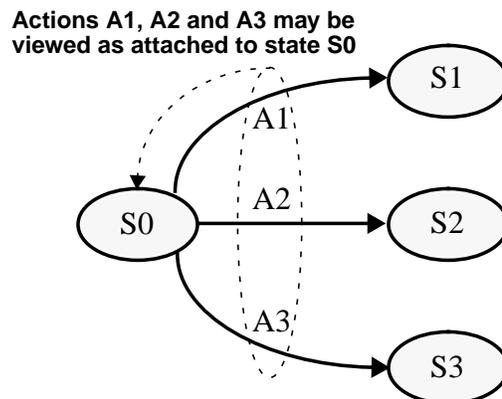
Figure 14. Actions may be viewed as attached to a state in a Mealy machine.
