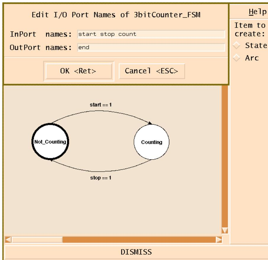
Figure 19. The FSM of the 3-bit counter.
